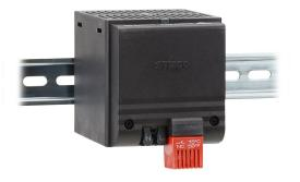
Stego enclosure heater, axial fan, 250W heating capacity, touchsafe PTC resistor heating element, 230 VAC operating voltage, 50/60 Hz, fixed thermostat, N.C. (open on rise) 41 deg F (5 deg C) switch-on, 35mm DIN rail mount.
