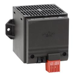
Stego enclosure heater, axial fan, 400W heating capacity, touch-safe PTC resistor heating element, 120 VAC operating voltage, 50/60 Hz, fixed thermostat, N.C. (open on rise) 41 deg F (5 deg C) switch-on, panel mount.
