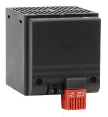
Stego enclosure heater, axial fan, 400W heating capacity, touchsafe PTC resistor heating element, 120 VAC operating voltage, 50/60 Hz, fixed thermostat, N.C. (open on rise) 41 deg F (5 deg C) switch-on, 35mm DIN rail mount.
