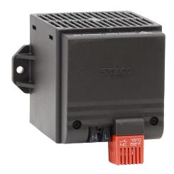
Stego enclosure heater, axial fan, 400W heating capacity, touch-safe PTC resistor heating element, 230 VAC operating voltage, 50/60 Hz, fixed thermostat, N.C. (open on rise) 41 deg F (5 deg C) switch-on, panel mount.
