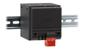
Stego enclosure heater, axial fan, 400W heating capacity, touchsafe PTC resistor heating element, 230 VAC operating voltage, 50/60 Hz, fixed thermostat, N.C. (open on rise) 41 deg F (5 deg C) switch-on, 35mm DIN rail mount.
