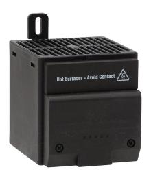
Stego enclosure heater, axial fan, 250W heating capacity, touchsafe PTC resistor heating element, 120 VAC operating voltage, 50/60 Hz, panel mount.
