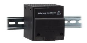
Stego enclosure heater, axial fan, 250W heating capacity, touch-safe PTC resistor heating element, 120 VAC operating voltage, 50/60 Hz, 35mm DIN rail mount.
