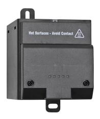
Stego enclosure heater, axial fan, 400W heating capacity, touchsafe PTC resistor heating element, 120 VAC operating voltage, 50/60 Hz, panel mount.
