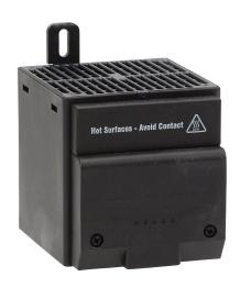
Stego enclosure heater, axial fan, 400W heating capacity, touch-safe PTC resistor heating element, 230 VAC operating voltage, 50/60 Hz, panel mount.
