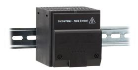
Stego enclosure heater, axial fan, 400W heating capacity, touch-safe PTC resistor heating element, 230 VAC operating voltage, 50/60 Hz, 35mm DIN rail mount.
