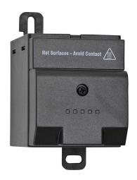
Stego enclosure heater, axial fan, 150W heating capacity, touchsafe PTC resistor heating element, 120 VAC operating voltage, 50/60 Hz, panel mount.
