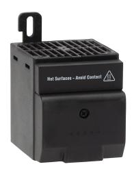
Stego enclosure heater, axial fan, 150W heating capacity, touch-safe PTC resistor heating element, 230 VAC operating voltage, 50/60 Hz, panel mount.
