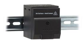
Stego enclosure heater, axial fan, 150W heating capacity, touch-safe PTC resistor heating element, 230 VAC operating voltage, 50/60 Hz, 35mm DIN rail mount.
