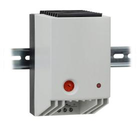
Stego enclosure heater, axial fan, 650W heating capacity, PTC resistor heating element, 100-120 VAC operating voltage, 50/60 Hz, adjustable thermostat, N.C. (open on rise) 0 to 60 deg C, 35mm DIN rail mount.
