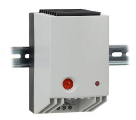
Stego enclosure heater, axial fan, 650W heating capacity, PTC resistor heating element, 100-120 VAC operating voltage, 50/60 Hz, adjustable thermostat, N.C. (open on rise) 0 to 60 deg C, 35mm DIN rail mount.
