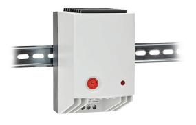
Stego enclosure heater, axial fan, 650W heating capacity, PTC resistor heating element, 100-120 VAC operating voltage, 50/60 Hz, adjustable thermostat, N.C. (open on rise) 32 to 140 deg F, 35mm DIN rail mount.
