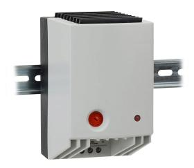
Stego enclosure heater, axial fan, 650W heating capacity, PTC resistor heating element, 220-240 VAC operating voltage, 50/60 Hz, adjustable thermostat, N.C. (open on rise) 0 to 60 deg C, 35mm DIN rail mount.
