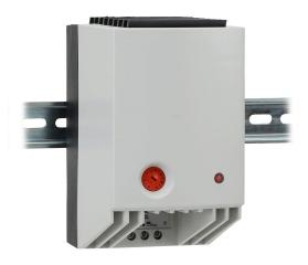
Stego enclosure heater, axial fan, 550W heating capacity, PTC resistor heating element, 100-120 VAC operating voltage, 50/60 Hz, adjustable thermostat, N.C. (open on rise) 0 to 60 deg C, 35mm DIN rail mount.
