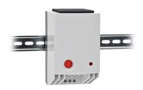
Stego enclosure heater, axial fan, 550W heating capacity, PTC resistor heating element, 100-120 VAC operating voltage, 50/60 Hz, adjustable thermostat, N.C. (open on rise) 32 to 140 deg F, 35mm DIN rail mount.
