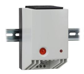
Stego enclosure heater, axial fan, 550W heating capacity, PTC resistor heating element, 220-240 VAC operating voltage, 50/60 Hz, adjustable thermostat, N.C. (open on rise) 0 to 60 deg C, 35mm DIN rail mount.
