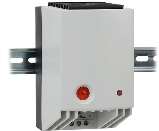
Stego enclosure heater, axial fan, 550W heating capacity, PTC resistor heating element, 220-240 VAC operating voltage, 50/60 Hz, adjustable thermostat, N.C. (open on rise) 0 to 60 deg C, 35mm DIN rail mount.
