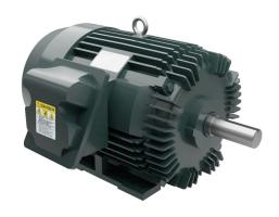
Toshiba SD premium efficiency AC induction motor, highperformance inverter duty and severe duty, 25hp, 3-phase, 230/460 VAC, 1200rpm, TEFC, NEMA 324T frame, cast iron, rigid base mount.
