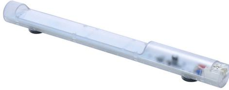
Stego Ecoline LED enclosure light, 24-48 VDC operating voltage, no switch, 13.8in length, 400 Lm, magnet mount, 2-pole dual cage clamp for 16 AWG stranded wire with ferrule or 14 AWG solid wire, 5W, IP20.
