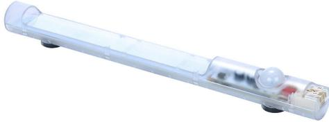
Stego Ecoline LED enclosure light, 100-240 VAC / 90-110 VDC operating voltage, motion sensor switch, 13.8in length, 400 Lm, magnet mount, 2-pole dual cage clamp for 16 AWG stranded wire with ferrule or 14 AWG solid wire, 5W, IP20.
