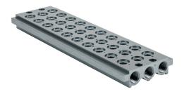
Metal Work air valve manifold, aluminum, silver, 145 psi (10 bar) maximum operating pressure, (10) stations, 3/8in female NPT inlet(s), 3/8in female NPT exhaust(s). For use with 1/4in NPT Series 70 valves.
