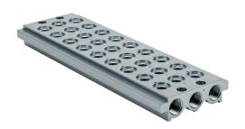
Metal Work air valve manifold, aluminum, silver, 145 psi (10 bar) maximum operating pressure, (9) stations, 3/8in female NPT inlet(s), 3/8in female NPT exhaust(s). For use with 1/4in NPT Series 70 valves.
