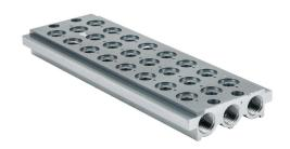
Metal Work air valve manifold, aluminum, silver, 145 psi (10 bar) maximum operating pressure, (8) stations, 3/8in female NPT inlet(s), 3/8in female NPT exhaust(s). For use with 1/4in NPT Series 70 valves.
