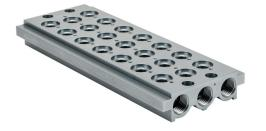
Metal Work air valve manifold, aluminum, silver, 145 psi (10 bar) maximum operating pressure, (7) stations, 3/8in female NPT inlet(s), 3/8in female NPT exhaust(s). For use with 1/4in NPT Series 70 valves.
