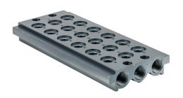
Metal Work air valve manifold, aluminum, silver, 145 psi (10 bar) maximum operating pressure, (6) stations, 3/8in female NPT inlet(s), 3/8in female NPT exhaust(s). For use with 1/4in NPT Series 70 valves.
