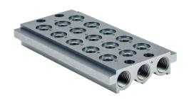
Metal Work air valve manifold, aluminum, silver, 145 psi (10 bar) maximum operating pressure, (5) stations, 3/8in female NPT inlet(s), 3/8in female NPT exhaust(s). For use with 1/4in NPT Series 70 valves.
