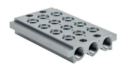
Metal Work air valve manifold, aluminum, 145 psi (10 bar) maximum operating pressure, (4) stations, 3/8in female NPT inlet(s), 3/8in female NPT exhaust(s). For use with 1/4in NPT Series 70 valves.
