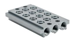
Metal Work air valve manifold, aluminum, silver, 145 psi (10 bar) maximum operating pressure, (4) stations, 3/8in female NPT inlet(s), 3/8in female NPT exhaust(s). For use with 1/4in NPT Series 70 valves.
