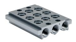
Metal Work air valve manifold, aluminum, silver, 145 psi (10 bar) maximum operating pressure, (3) stations, 3/8in female NPT inlet(s), 3/8in female NPT exhaust(s). For use with 1/4in NPT Series 70 valves.
