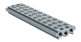
Metal Work air valve manifold, aluminum, 145 psi (10 bar) maximum operating pressure, (10) stations, 1/4in female NPT inlet(s), 1/4in female NPT exhaust(s). For use with 1/8in NPT Series 70 valves.
