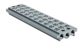
Metal Work air valve manifold, aluminum, silver, 145 psi (10 bar) maximum operating pressure, (10) stations, 1/4in female NPT inlet(s), 1/4in female NPT exhaust(s). For use with 1/8in NPT Series 70 valves.
