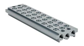
Metal Work air valve manifold, aluminum, silver, 145 psi (10 bar) maximum operating pressure, (9) stations, 1/4in female NPT inlet(s), 1/4in female NPT exhaust(s). For use with 1/8in NPT Series 70 valves.
