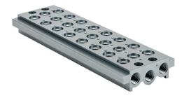
Metal Work air valve manifold, aluminum, silver, 145 psi (10 bar) maximum operating pressure, (8) stations, 1/4in female NPT inlet(s), 1/4in female NPT exhaust(s). For use with 1/8in NPT Series 70 valves.
