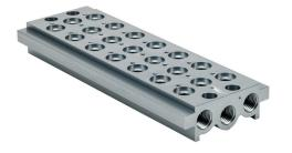
Metal Work air valve manifold, aluminum, silver, 145 psi (10 bar) maximum operating pressure, (7) stations, 1/4in female NPT inlet(s), 1/4in female NPT exhaust(s). For use with 1/8in NPT Series 70 valves.
