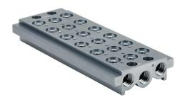
Metal Work air valve manifold, aluminum, silver, 145 psi (10 bar) maximum operating pressure, (6) stations, 1/4in female NPT inlet(s), 1/4in female NPT exhaust(s). For use with 1/8in NPT Series 70 valves.
