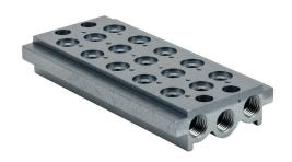
Metal Work air valve manifold, aluminum, silver, 145 psi (10 bar) maximum operating pressure, (5) stations, 1/4in female NPT inlet(s), 1/4in female NPT exhaust(s). For use with 1/8in NPT Series 70 valves.
