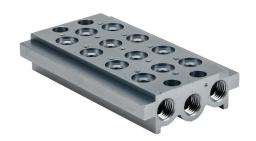
Metal Work air valve manifold, aluminum, silver, 145 psi (10 bar) maximum operating pressure, (4) stations, 1/4in female NPT inlet(s), 1/4in female NPT exhaust(s). For use with 1/8in NPT Series 70 valves.
