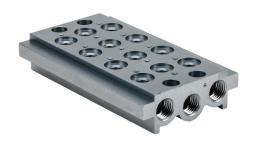
Metal Work air valve manifold, aluminum, 145 psi (10 bar) maximum operating pressure, (4) stations, 1/4in female NPT inlet(s), 1/4in female NPT exhaust(s). For use with 1/8in NPT Series 70 valves.
