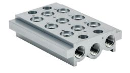
Metal Work air valve manifold, aluminum, silver, 145 psi (10 bar) maximum operating pressure, (3) stations, 1/4in female NPT inlet(s), 1/4in female NPT exhaust(s). For use with 1/8in NPT Series 70 valves.
