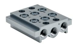
Metal Work air valve manifold, aluminum, silver, 145 psi (10 bar) maximum operating pressure, (2) stations, 1/4in female NPT inlet(s), 1/4in female NPT exhaust(s). For use with 1/8in NPT Series 70 valves.
