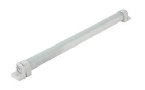
Stego Varioline LED enclosure light, 100-240 VAC operating voltage, no switch, 23.4in length, 1730 Lm, magnet mount, 2-pole plug with snap lock, 16W, IP20.
