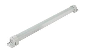
Stego Varioline LED enclosure light, 100-240 VAC operating voltage, motion sensor switch, 23.4in length, 1730 Lm, screw mount, 2-pole plug with snap lock, 16W, IP20.
