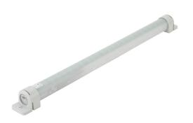
Stego Varioline LED enclosure light, 100-240 VAC operating voltage, on/off switch, 23.4in length, 1730 Lm, magnet mount, 2-pole plug with snap lock, 16W, IP20.
