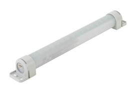
Stego Varioline LED enclosure light, 100-240 VAC operating voltage, no switch, 15.6in length, 1080 Lm, screw mount, 2-pole plug with snap lock, 11W, IP20.
