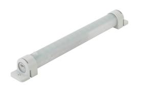
Stego Varioline LED enclosure light, 100-240 VAC operating voltage, motion sensor switch, 15.6in length, 1080 Lm, magnet mount, 2-pole plug with snap lock, 11W, IP20.
