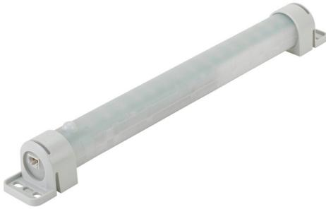
Stego Varioline LED enclosure light, 100-240 VAC operating voltage, motion sensor switch, 15.6in length, 1080 Lm, screw mount, 2-pole plug with snap lock, 11W, IP20.
