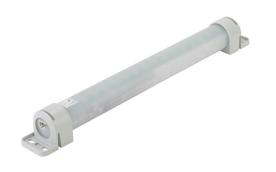
Stego Varioline LED enclosure light, 100-240 VAC operating voltage, on/off switch, 15.6in length, 1080 Lm, screw mount, 2-pole plug with snap lock, 11W, IP20.
