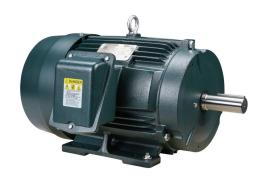
Toshiba SD premium efficiency AC induction motor, high-performance inverter duty and severe duty, 20hp, 3-phase, 230/460 VAC, 1800rpm, TEFC, NEMA 256T frame, cast iron, rigid base mount.
