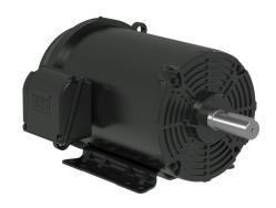
WEG Electric S premium efficiency AC induction motor, general purpose and inverter rated, 20hp, 3-phase, 208-230/460 VAC, 3600rpm, TEFC, NEMA 256T frame, rolled steel, rigid base mount.
