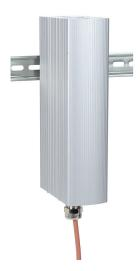
Stego enclosure heater, hazardous location rated, 200W heating capacity, high performance cartridge heating element, 120 VAC operating voltage, 35mm DIN rail mount.
