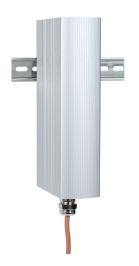
Stego enclosure heater, hazardous location rated, 200W heating capacity, high performance cartridge heating element, 230 VAC operating voltage, 35mm DIN rail mount.
